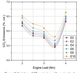
Figure 9. Variation of CO<sub>2</sub> emission with engine load
