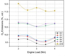
Figure 10. Variation of O<sub>2</sub> emission with engine load
