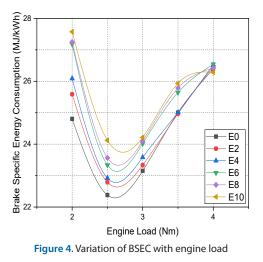
gy released in the cylinder decreased and fuel consumption increased with bioethanol usage, and therefore BSEC values increased.
