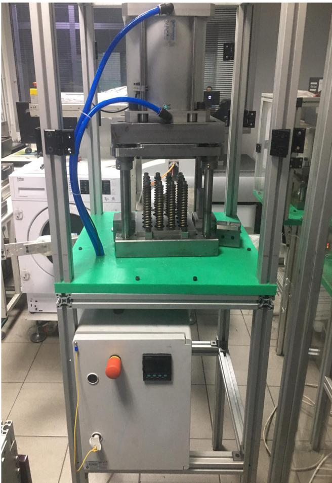
**Figure 7.** Compression spring fatigue machine.
