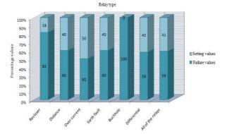
Figure 5. The incorrect percentage values all of the relays
