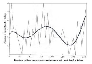
Figure 8. The number of circuit breaker failures over time after previous preventive maintenance
