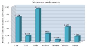
Figure 6. The performance of transformers in the NAEPN according to their producer company
