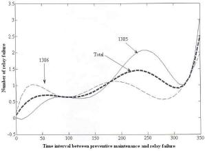
Figure 7. Relation between the numbers of relays failures and the time interval from the previous preventive maintenance
