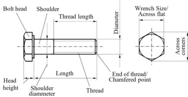
Figure 5. Parts of hex head bolt [26]
