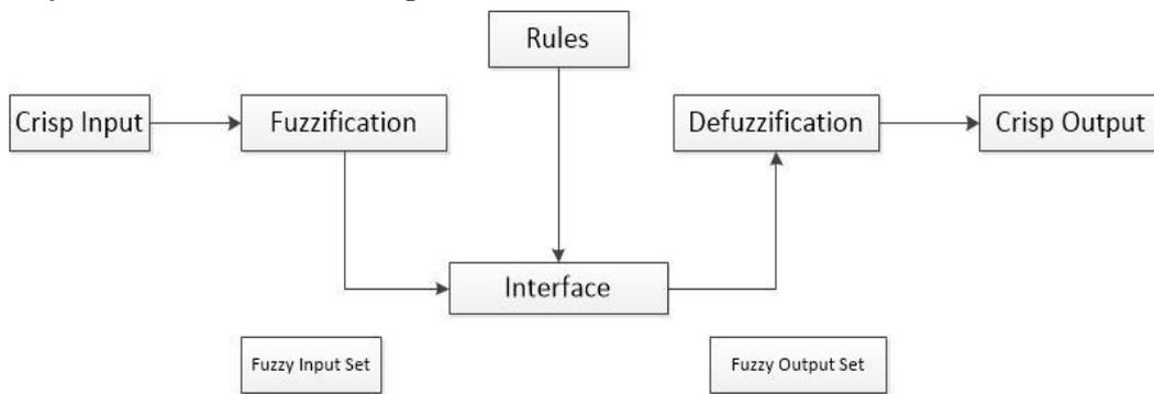
**Figure 1.** General structure of fuzzy logic system (Mendel, 1995).
