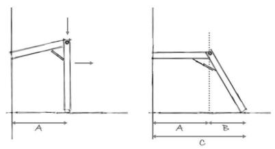
Figure 13. Abstracted movement mechanism (closed - open) [21]
