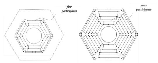
Figure 15. Capacity change plan scheme in auditorium design (closed-open) [21]
