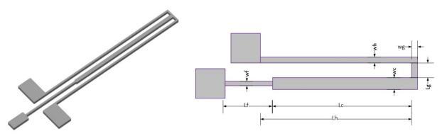
Figure 3: a) CAD design of the actuator, b) Dimensioning of the Electro-Thermal Actuator with symmetrical structure.
