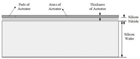
Figure 4: Printing the Elecro Thermal Actuator on the silicon wafer
