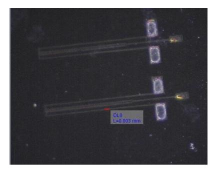
Figure 5: Top view of fabricated Electro-Thermal Actuator obtained by 3D printer camera
