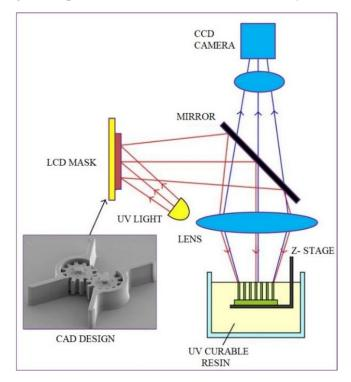
Figure 1: PµSL working principle [21].
