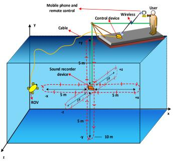
Fig. 2. Experimental setup for direction underwater sounds acquisition
