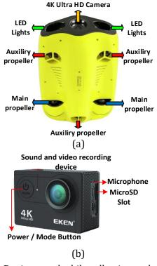
Fig. 1. Devices used while collecting underwater direction dataset (a) Underwater robot (b) Sound and video recording device
