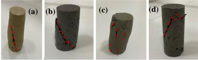
Figure 6 UCS test of clay mixture with various fly ash contents (a) clay mixture, (b) C+10% FA, (c) C+15% FA and (d) C+20% FA
