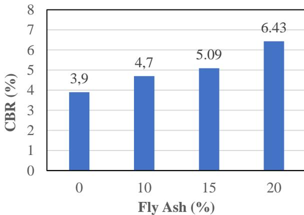
Figure 9 CBR values (%) vs. fly ash content (%)
