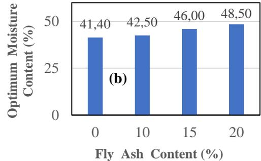
Figure 5 (a) The variation of maximum dry density ( $\text{g/cm}^3$ ) with fly ash content (%), (b) the variation of optimum moisture content (%) with fly ash content (%)
