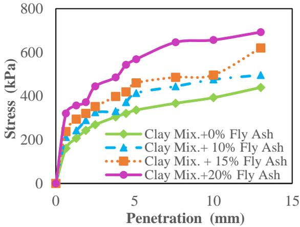
Figure 8 CBR Test results: Stress (kPa) versus Penetration (mm)
