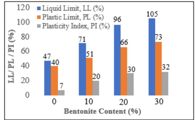
Figure 2 Liquid Limit (LL) (%), Plastic Limit (PL) (%) and (c) Plasticity Index (PI) (%) values for K, 90K+10B, 80K+20B, and 70K+30B
