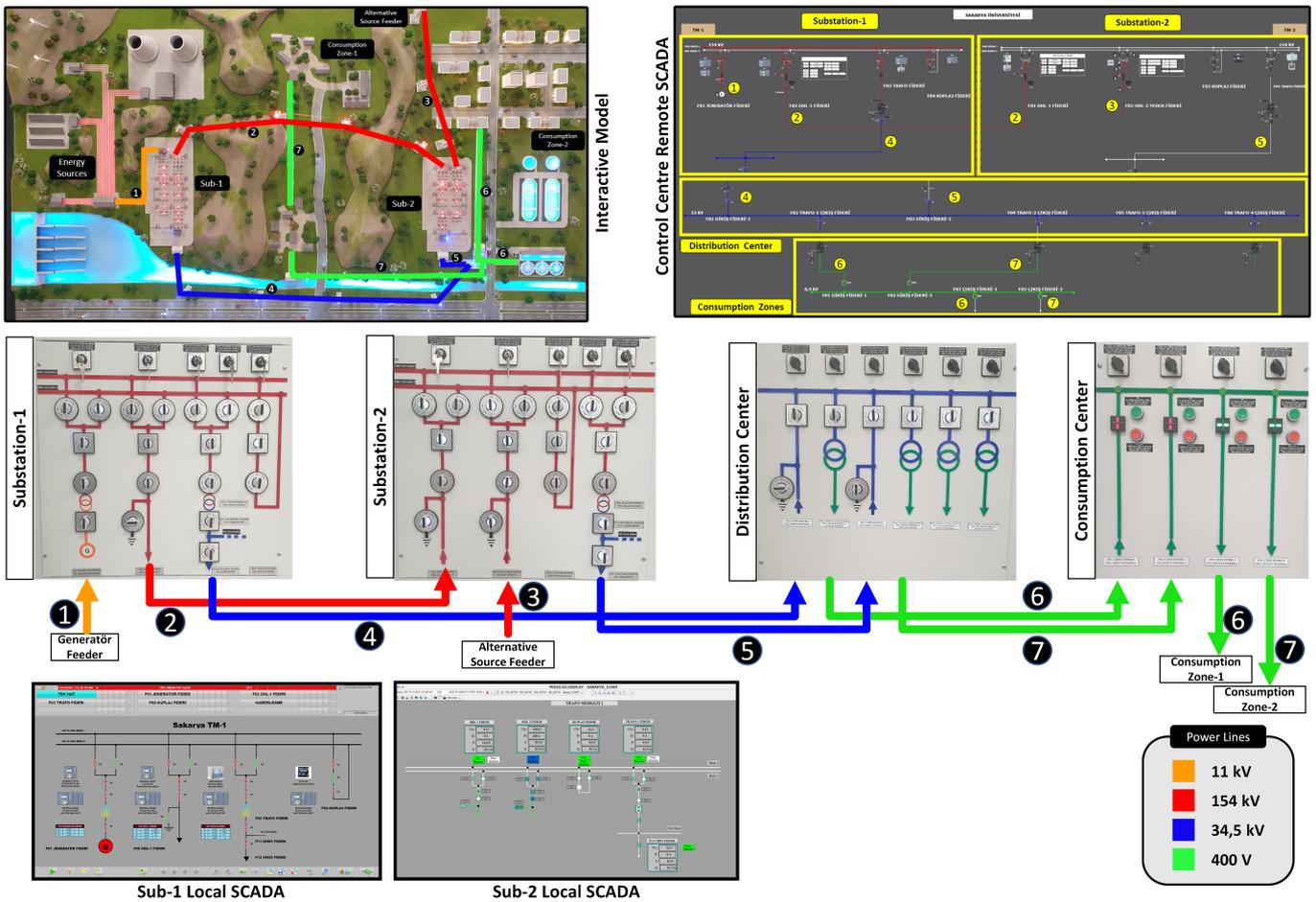
Figure 2. Process Architecture Topology of The Electric Energy Management Testbed Center.
