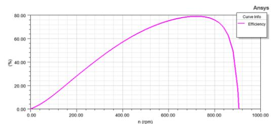
Figure 8. The efficiency-speed curves of the designed machine.
