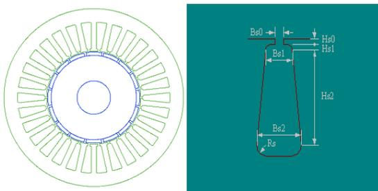
Figure 2. General view of the designed motor structure and slot type.
