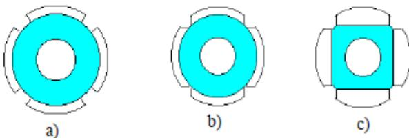
**Figure 1.** Different rotor structures of the surface magnet PM motor; a) surface magnets perpendicular to the rotor shaft, b) surface magnets parallel to the rotor shaft, c) bread-shaped magnets.
