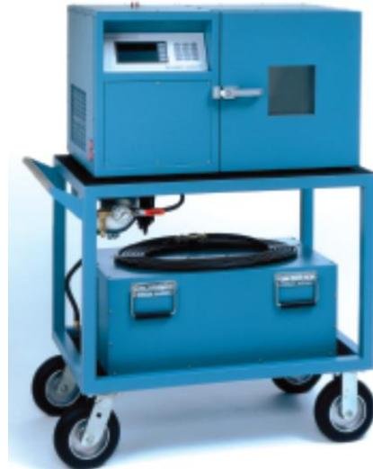
**Figure 1.** The two-pressure humidity generator
