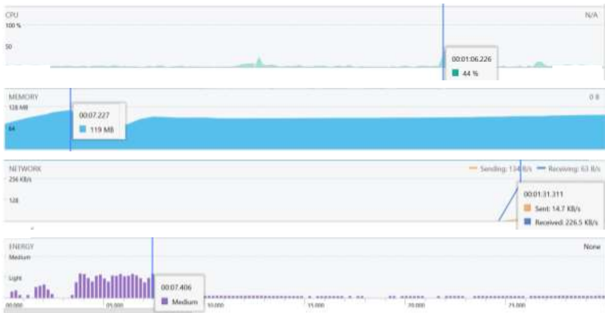
Fig. 3. Performance test results show the application’s maximum usage of the device’s CPU, memory, network, and energy.
