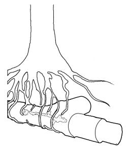
Figure 3. Infiltration of roots into cracks (developed by Author C. Korkmaz, 2023)
