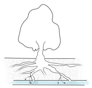
Figure 5. Roots directed towards the pipe (developed by Author C. Korkmaz, 2023)
