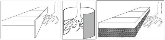
Figure 7. Linear, circular and three-dimensional root barriers (Morgenroth, 2008)
