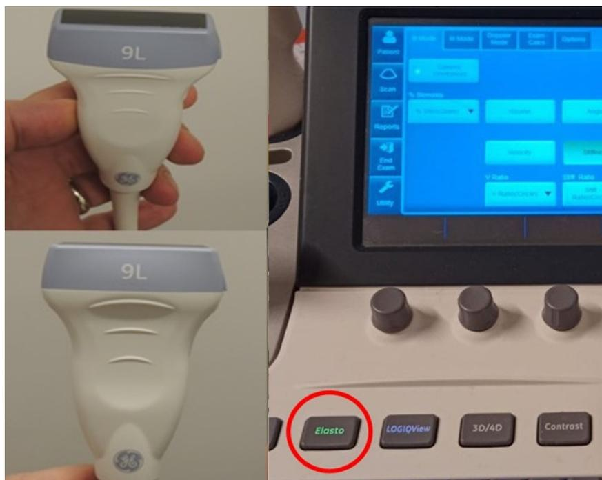
**Fig. 1.** Touch panel and button panel of GE Logic S8 brand/model USG device with elastography software (elastography button is circled in red on the right) and a 9 Mhz linear probe with hardware elastography features (shown from two different directions on the left).
