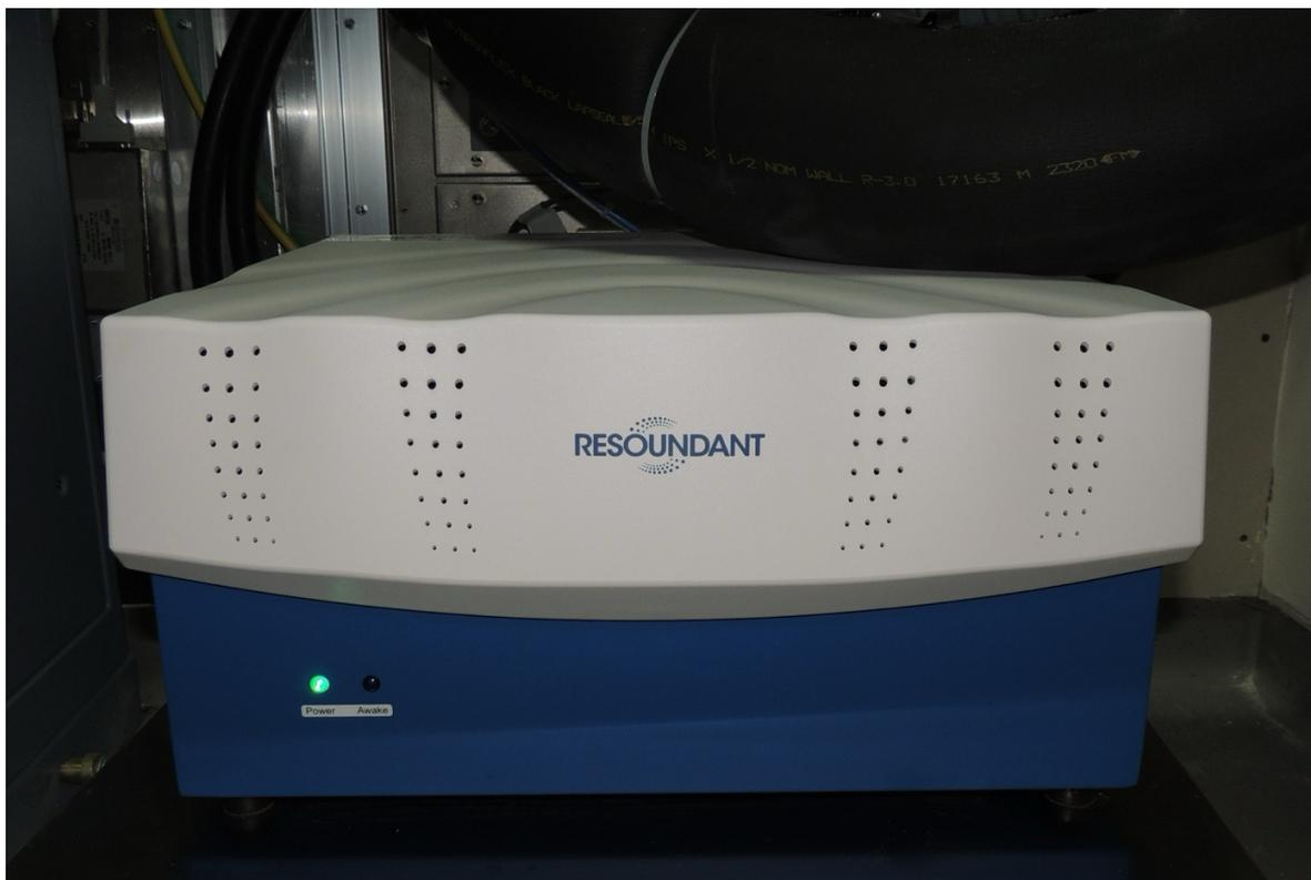
**Fig. 4.** The so-called "active driver", which is an additional component of the MRE examination, is shown.
